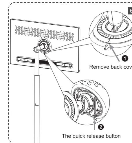
**Attention: To disassemble, press the quick release button.**
